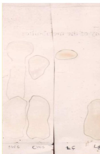
FIG. 6: Thin layer chromatography of the metabolites (spot locations) of IWS,CWS and LC using petroleum ether/diethyl ether/glacial acetic acid (90:10:1 by vol) as solvent.
