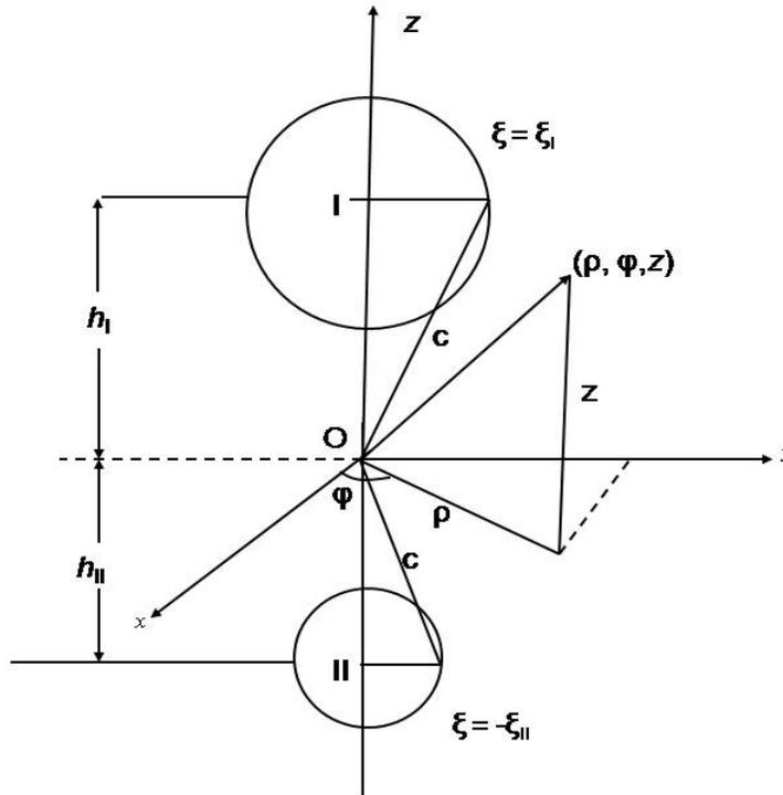
Figure 1 Schematic diagram of the geometry of two sphere problem.
