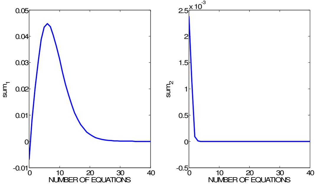
Figure 2 A plot of the convergence test using equations  $\{sum_1\}$  and  $\{sum_2\}$  against the number of equations for sphere sizes  $R_I$  and  $R_{II} = 0.5 \times 10^{-3}, 10^{-4}$  m respectively, with the following translational velocities  $U_y^I = 3 \times 10^{-3}$ ,  $U_y^{II} = 0$  m s $^{-1}$ . (a) Represent the calculation of the sum of the coefficients using equation 4.8. (b) Represent the calculation of the sum of the coefficients using equation 4.9.
